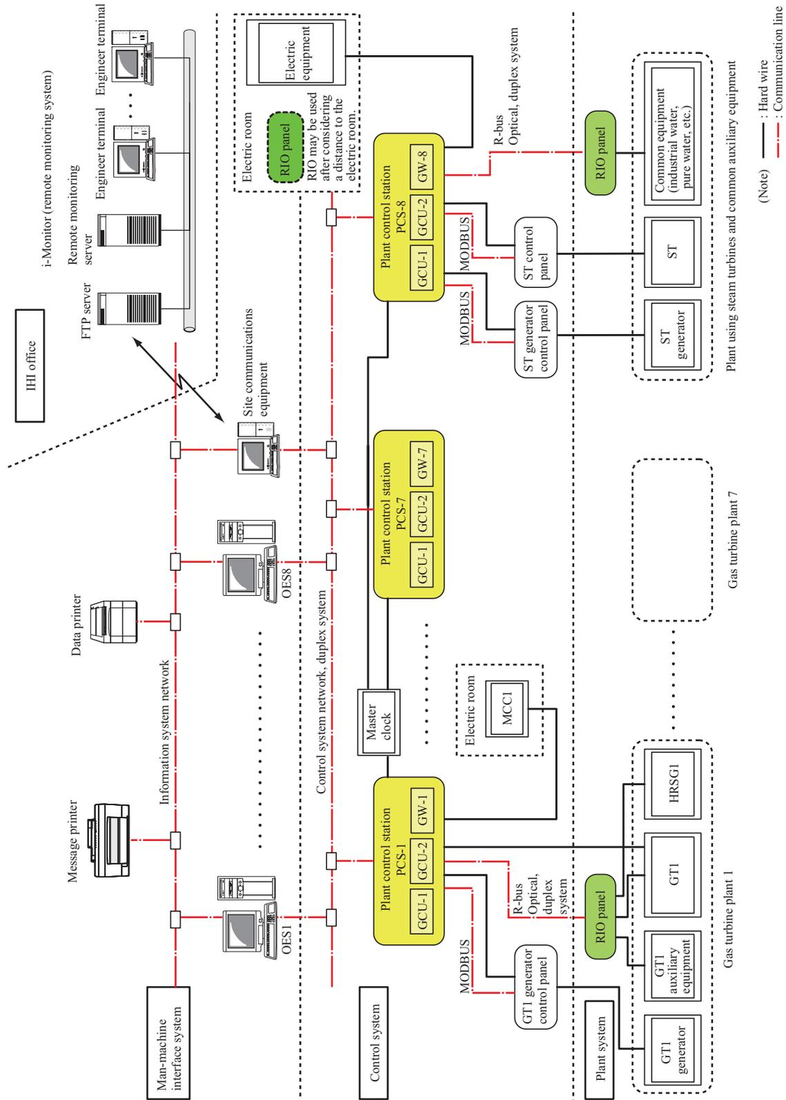
Fig. 1 Control system configuration of gas turbine power plants
