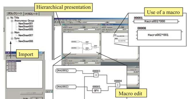
Fig. 4 Control logic editor (LogiCAD)
