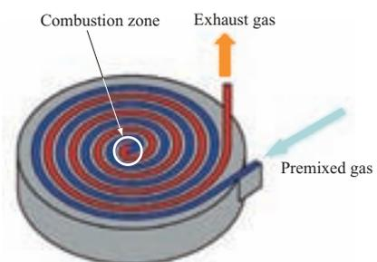
Fig. 2 Swiss-roll type micro combustor
