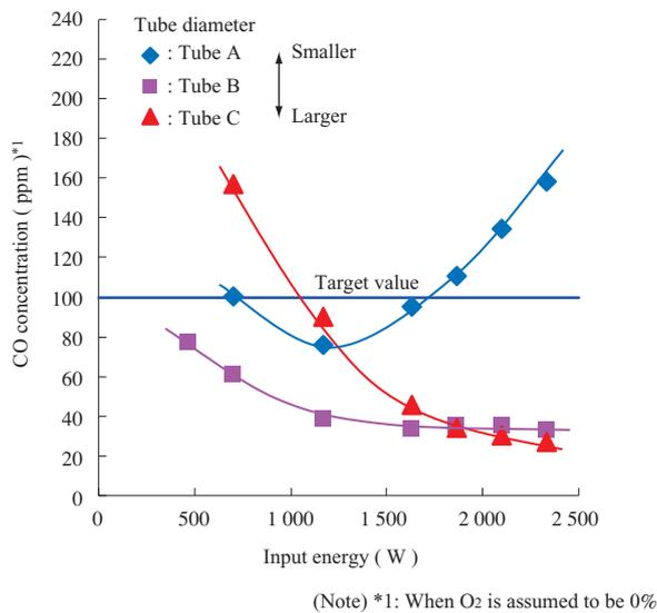
Fig. 8 Effect of outer-tube diameter on CO concentration
