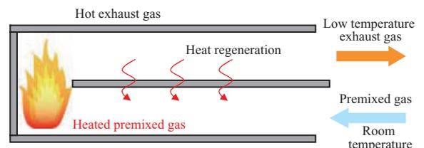
Fig. 1 Mechanism of excess enthalpy combustion
