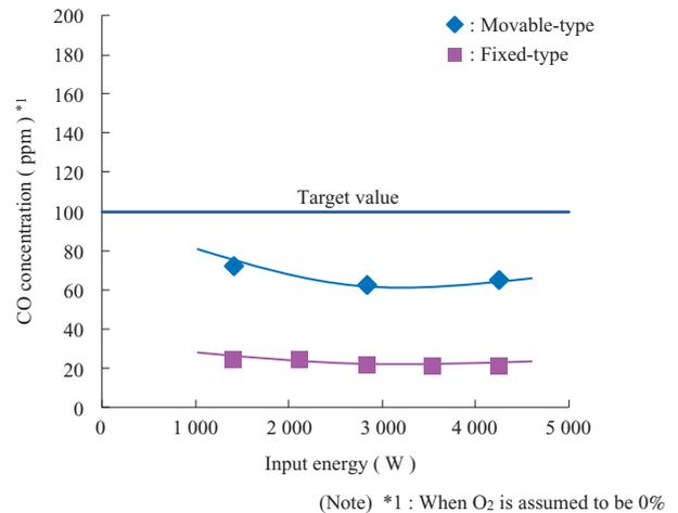
Fig. 11 Exhaust CO concentration in prototype commercial unit test
