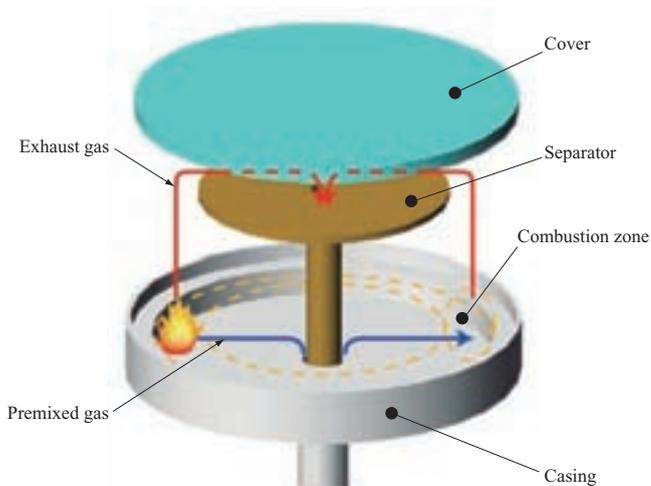
Fig. 3 Disk-type micro combustor
