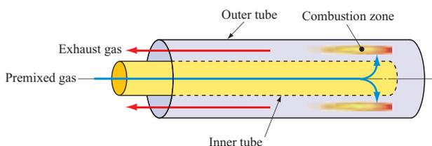
Fig. 5 Tube-type micro combustor
