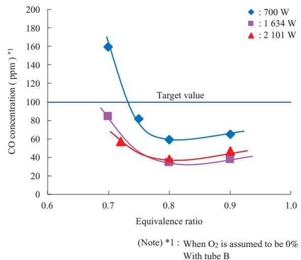
Fig. 9 Effect of equivalence ratio on CO concentration
