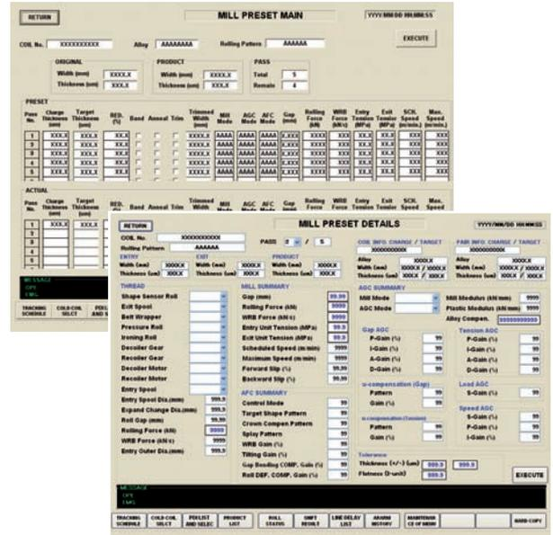
Fig. 1 Interface samples for aluminum foil mill setting calculation system
