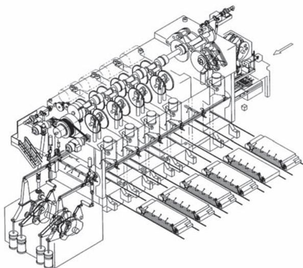
Fig. 8 Feeding system of the transfer press
