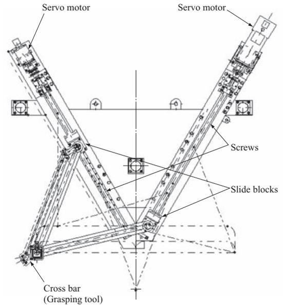
Fig. 9 Outline of high speed feeding system
