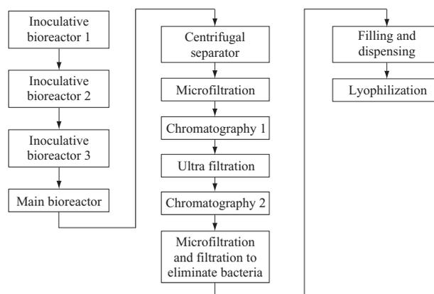
Fig. 1 Biopharmaceutical manufacturing process
