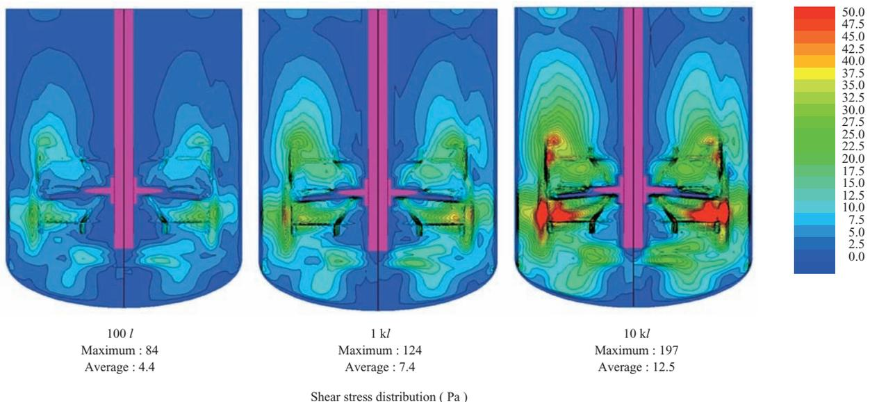
**Fig. 7** Shear stress distribution in bioreactor
