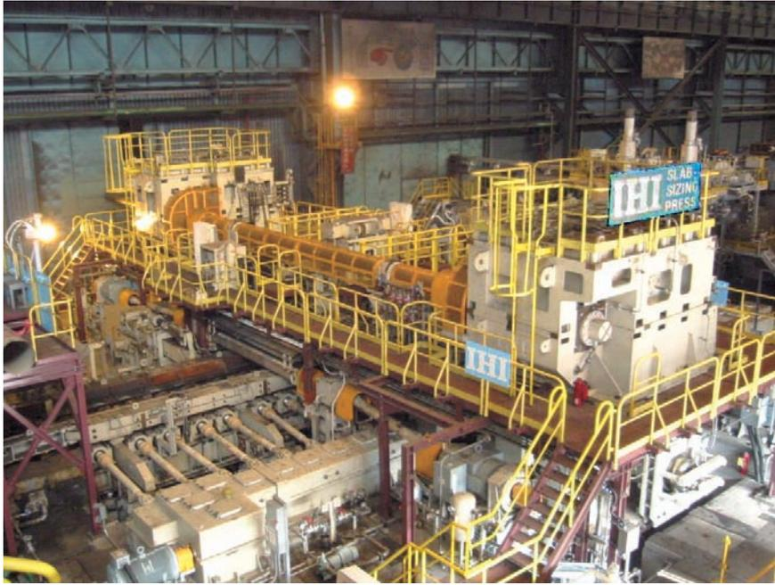
Fig. 2 Slab-width sizing press
