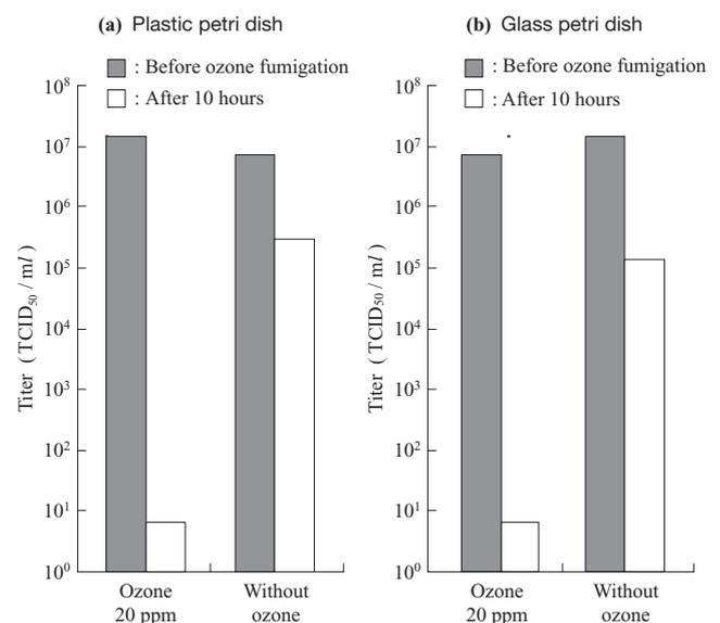
Fig. 3 Inactivation of influenza virus attached to carrier surfaces
