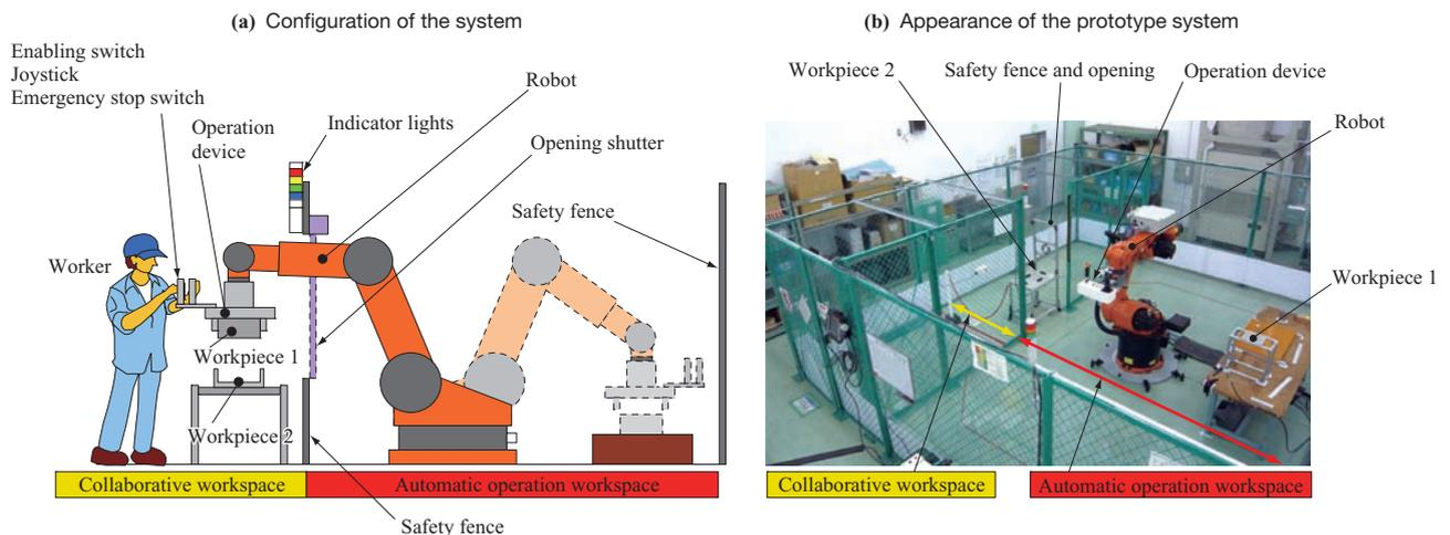
Fig. 3 Concept of hand guiding system
