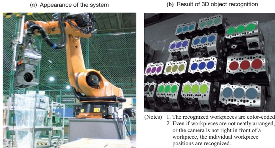
Fig. 2 Medium payload handling robot
