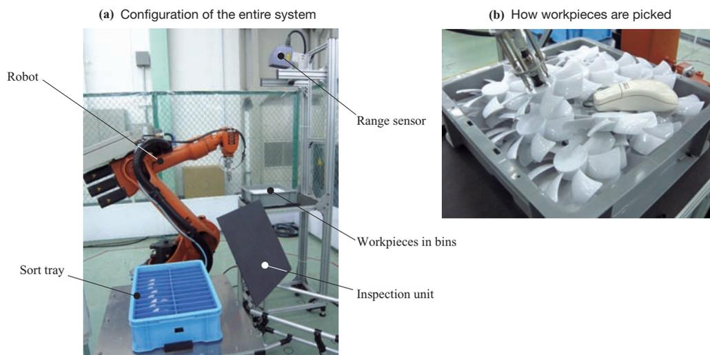
Fig. 1 Bin picking robotics using 3D object recognition
