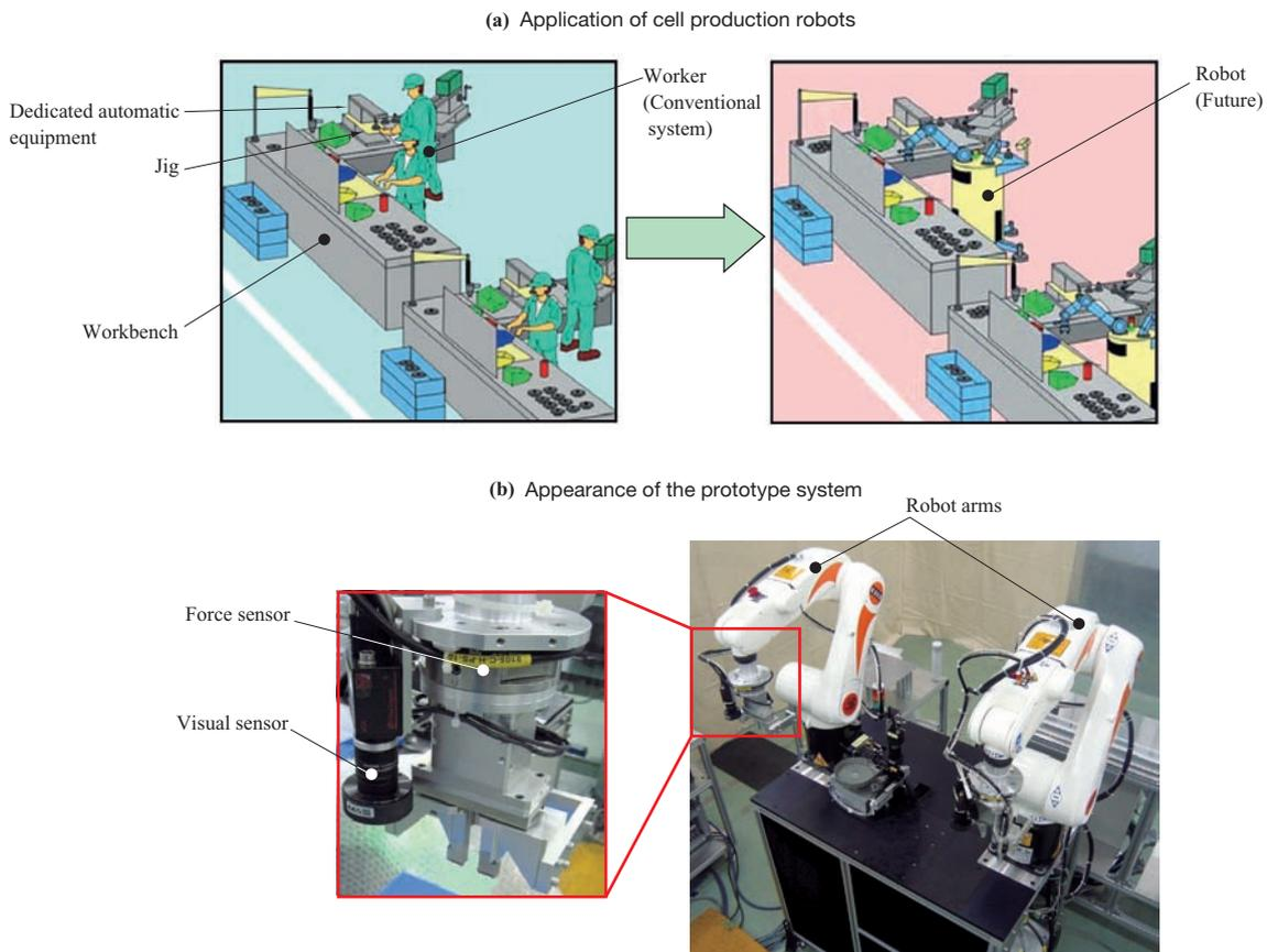
Fig. 4 Cell production robot system
