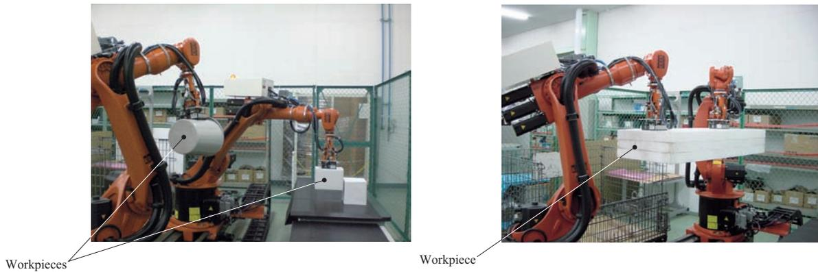
Fig. 5 Cooperative handling robots
