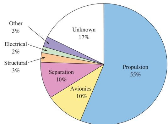
Fig. 5 Launch vehicle subsystem failures (1980-1999)
