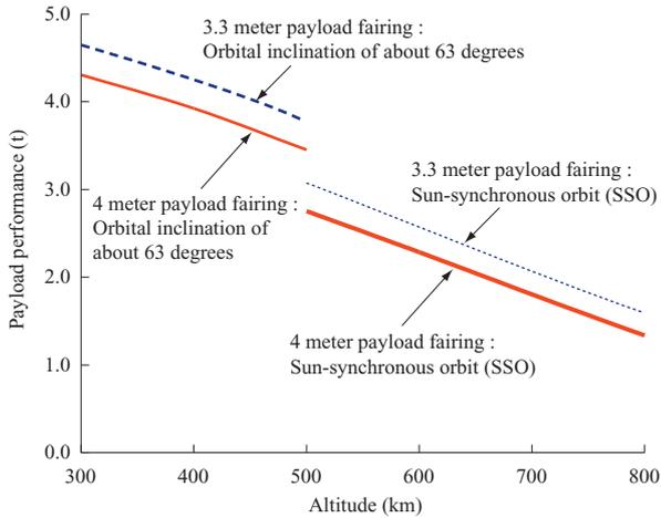
Fig. 8 Payload performance of the GX launch vehicle
