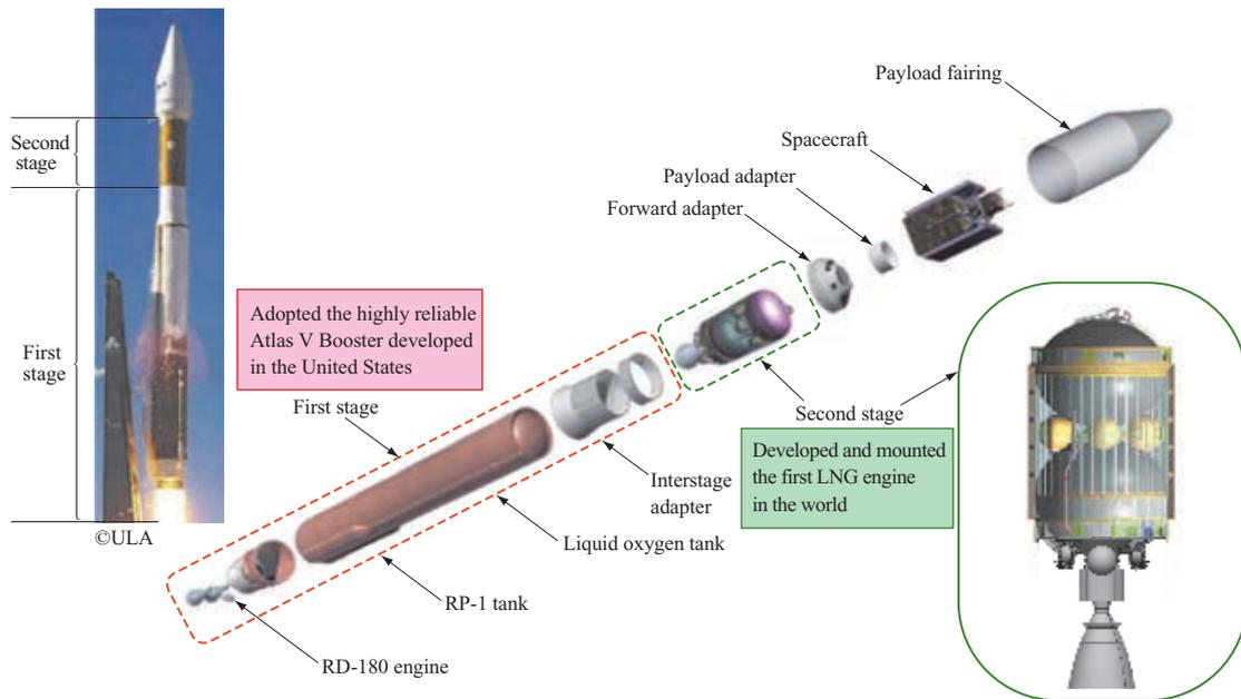
Fig. 2 Major components of the GX launch vehicle
