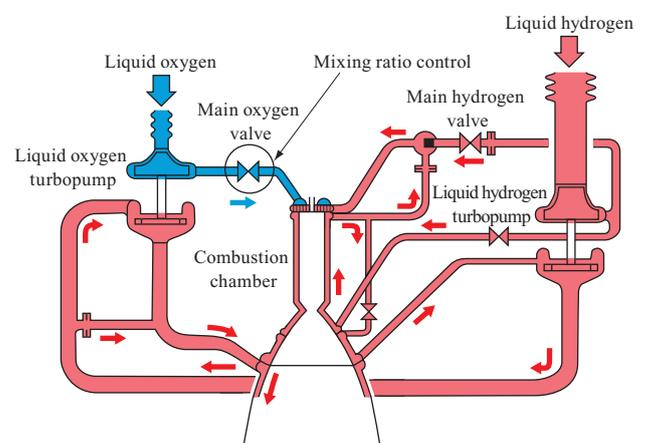
Fig. 2 LE-X engine cycle
