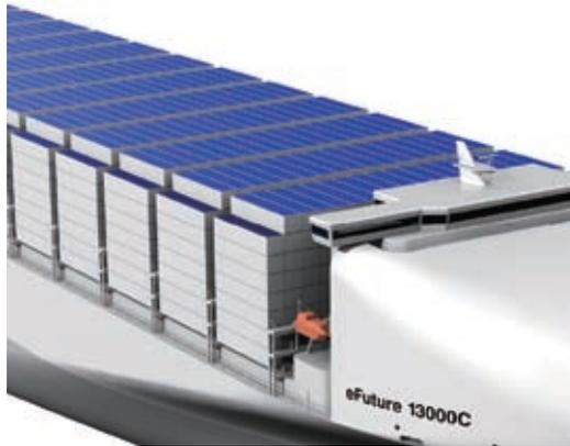
Fig. 10 Arrangement of photovoltaic panels
