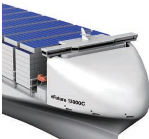
Fig. 6 Forward bridge and front bonnet
