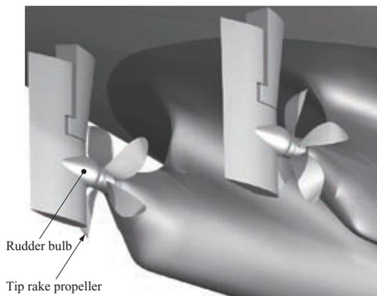
Fig. 5 Tip rake propeller and rudder bulb
