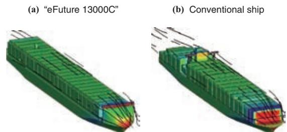
Fig. 8 Air flow and pressure distribution around ship by CFD analysis
