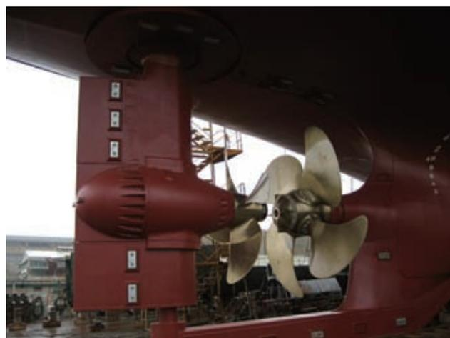
Tandem contra-rotating propeller, rudder propeller (ZP-41RP)
