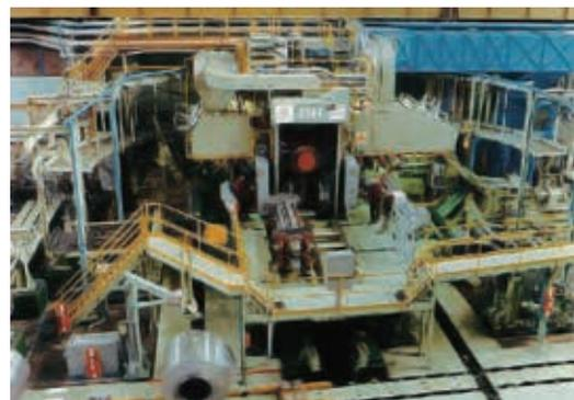
Fig. 6 Aluminum single stand cold rolling mill
