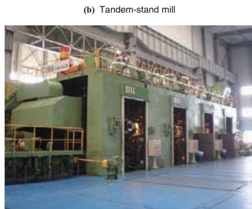
**Fig. 3** Aluminum hot rolling mill
