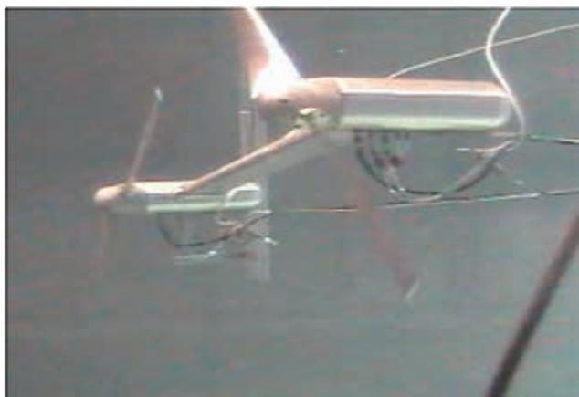
Tank experiment using scale model of floating turbine
