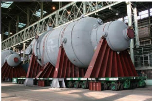
Tubular reactor, a typical product of Yokohama Nuclear & Chemical Components Works
