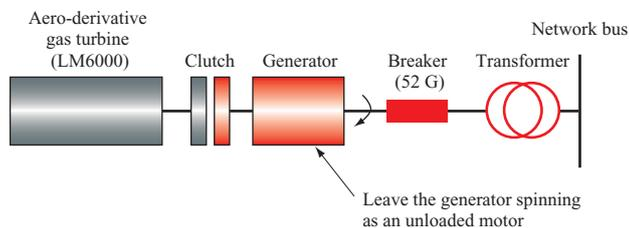
Fig. 3 Clutch-coupled configuration of spinning reserve
