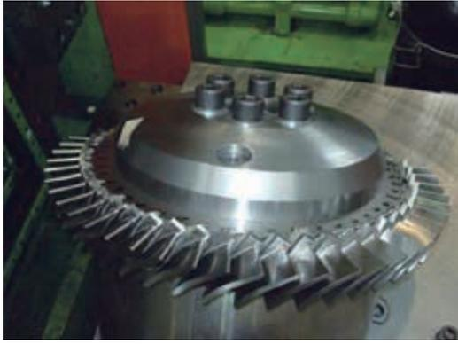
Fig. 10 Compressor blisk manufactured by LFW<sup>(3)</sup>
