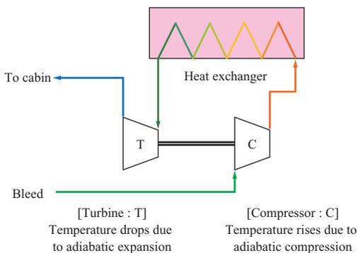
Fig. 2 Outline of air-conditioning using ACS
