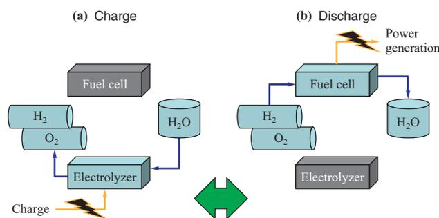
**Fig. 4** Charge and discharge behavior of on-board RFC
