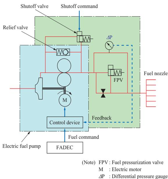
Fig. 5 Schematic of electrical fuel system
