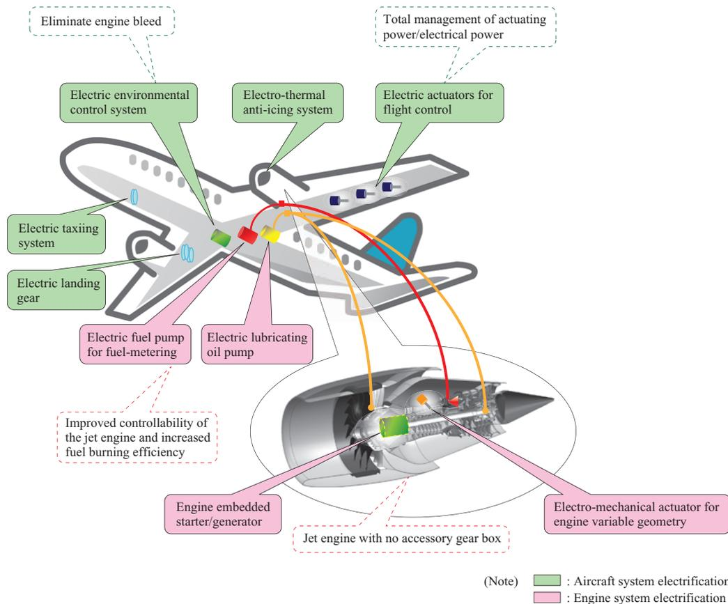
Fig. 1 Overview of the All-Electric Aircraft system
