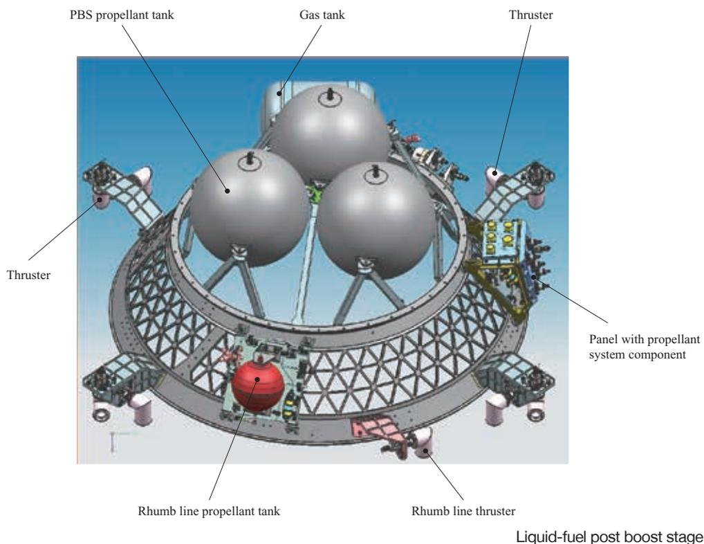
propellant rocket, it has become possible in the final stage to perform fine adjustment for placing a satellite into orbit.
