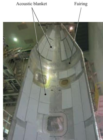
Lessening the satellite environment (vibration suppression mechanism, acoustic blanket)
