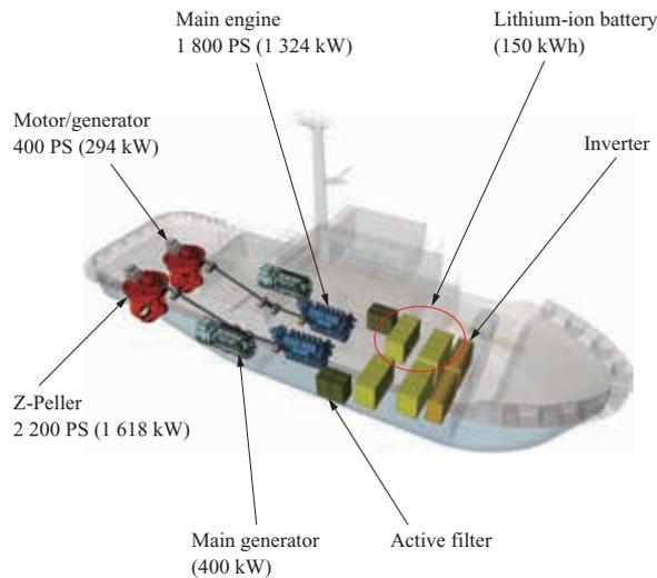
Fig. 8 Layout and capacity of the hybrid tugboat
