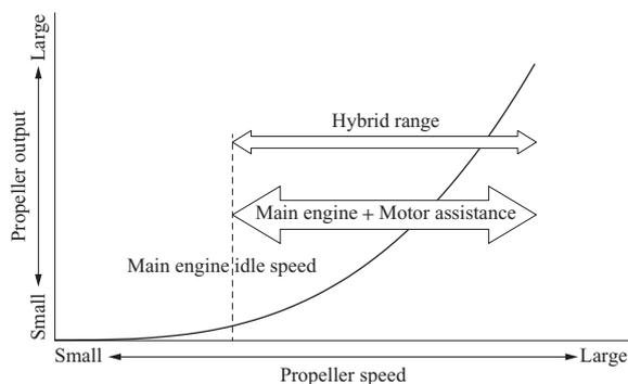
Fig. 5 Work mode (Bollard-Pull mode)
