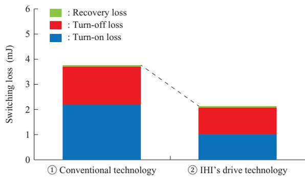
(Note) The loss is around 18 mJ with a silicon IGBT as a conventional device (according to IHI's evaluation).
