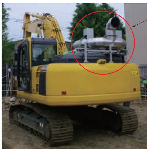
Installed active silencer (Prototype)
