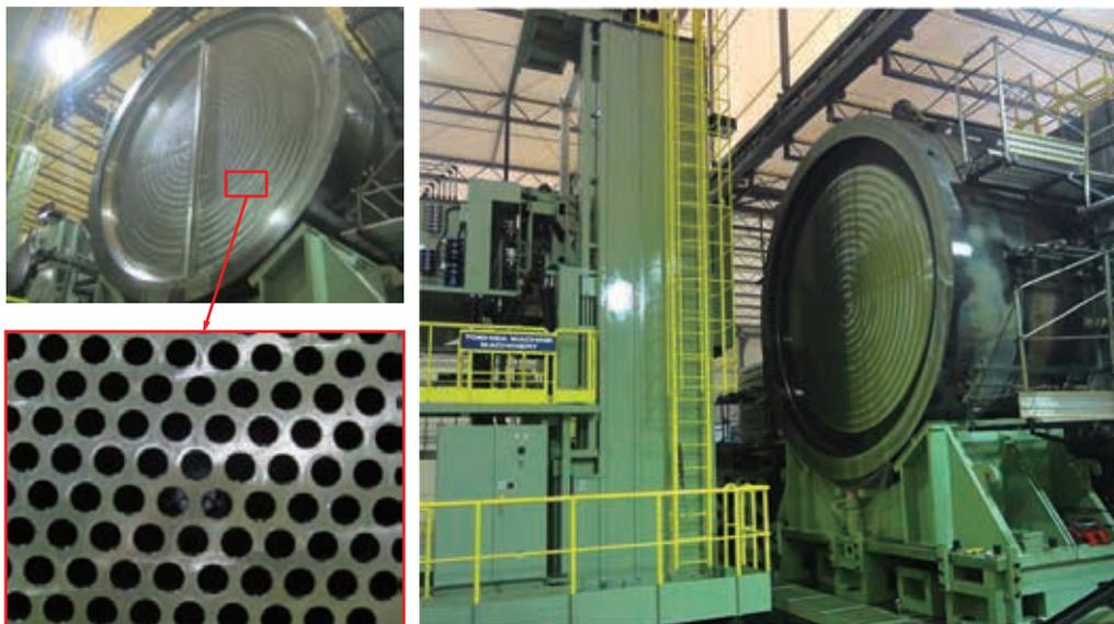
Deep hole-drilling machine for tube sheet BTA (Boring and Trepanning Association)
