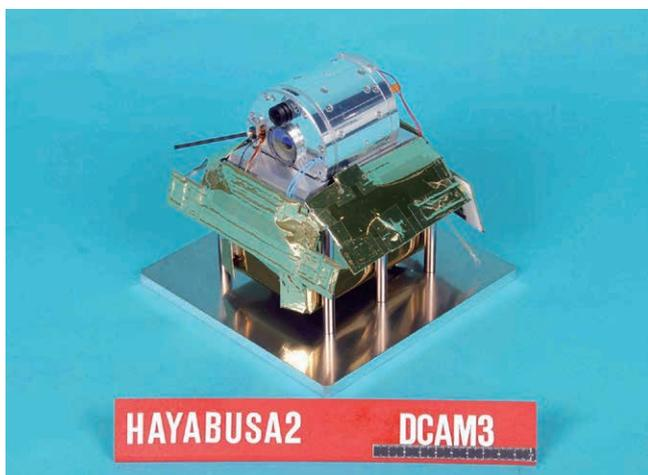
Separation Camera DCAM3 ©JAXA
