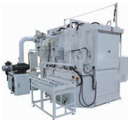
Exterior view of batch-type vacuum carburizing equipment (VCB)
