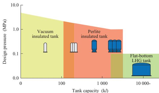
Scope of application of above-ground LNG storage tanks
