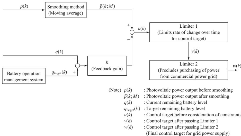
Fig. 2 Calculation model of the control target supplying power to the commercial power grid
