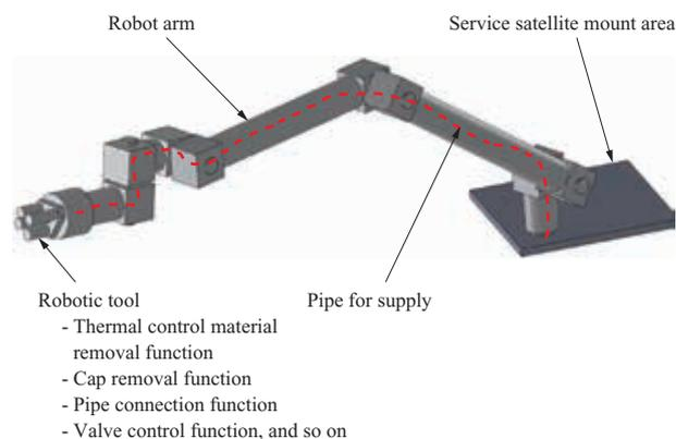
Conceptual diagram of robot arm for on-orbit satellite services
