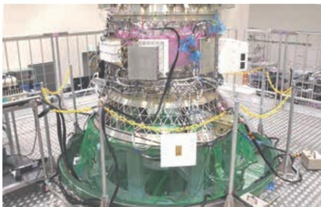
PSDB assembled in three-stage device mount structure
