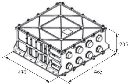
Relay-based PSDB (Test vehicle)
