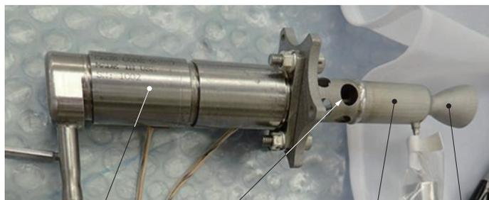
Valve      Supply piping part      Combustion chamber      Nozzle
