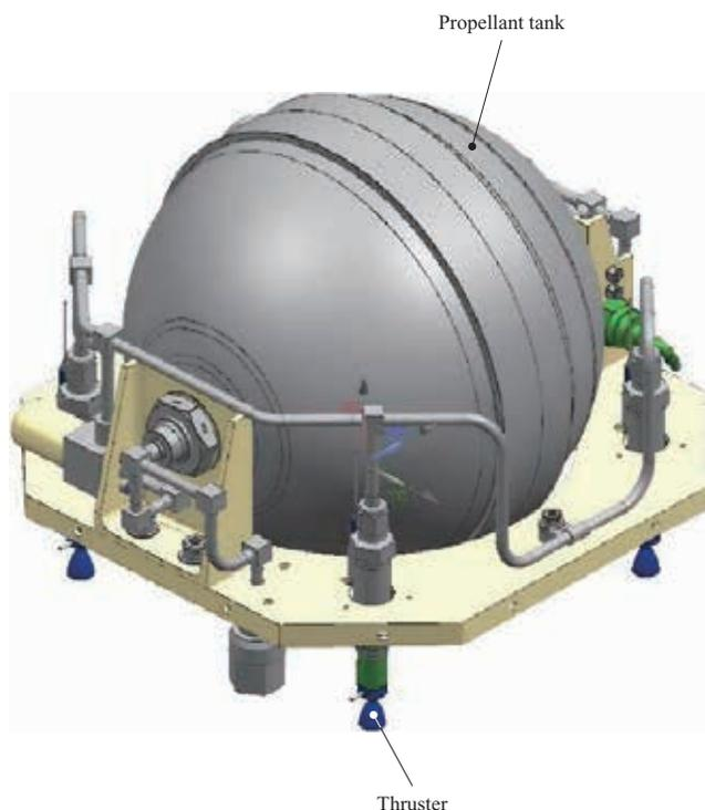
Schematic diagram of propulsion unit
