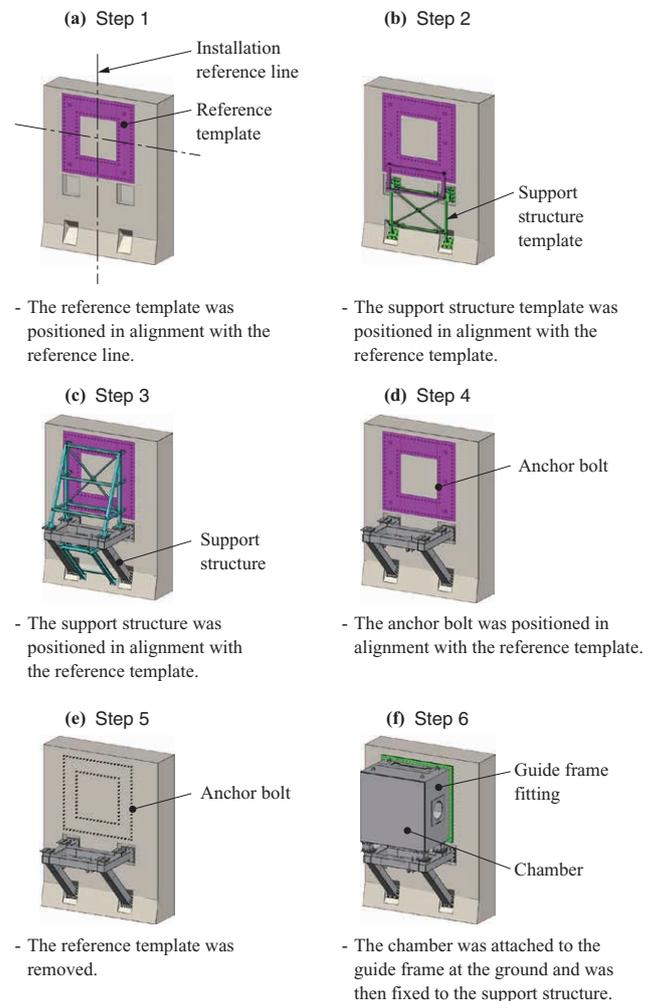
Fig. 2 Installation procedure using the original steel templates
