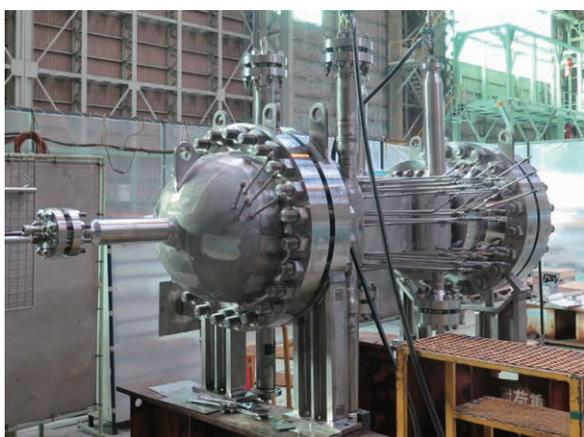
Compact reactor capable of producing 8 000 Nm<sup>3</sup>/d of hydrogen
