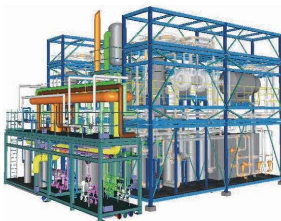
Example of modularized plant with two compact reactor systems
