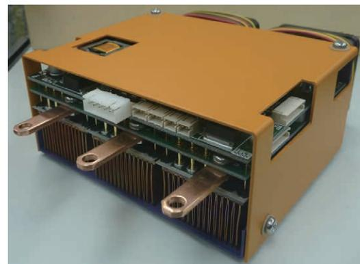
Fig. 11 Prototype of high power-density SiC inverter
