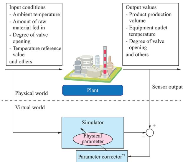
(Note) \*1 : The physical parameters in the simulator are adjusted sequentially so that the input and output values are consistent with the actual sensor values.
