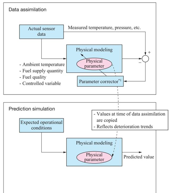
(Note) \*1 : The physical parameters in the simulator are adjusted sequentially so that the input and output values are consistent with the actual sensor values.
