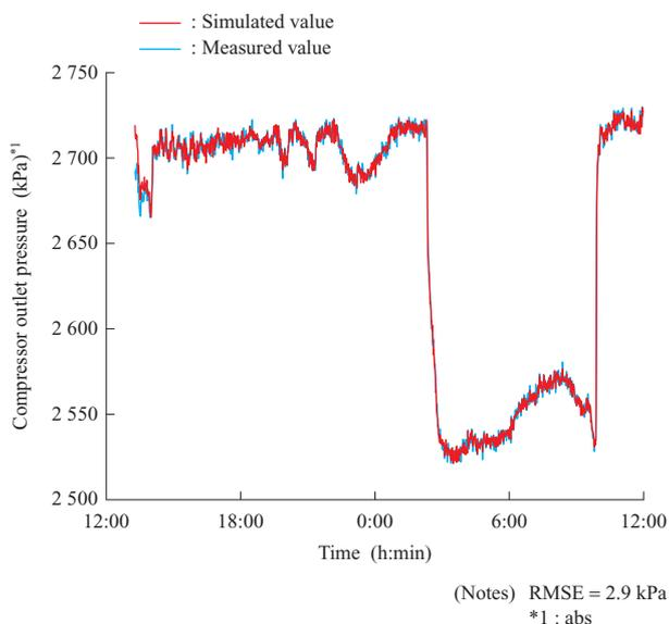
Fig. 6 Simulated and measured values during data assimilation
