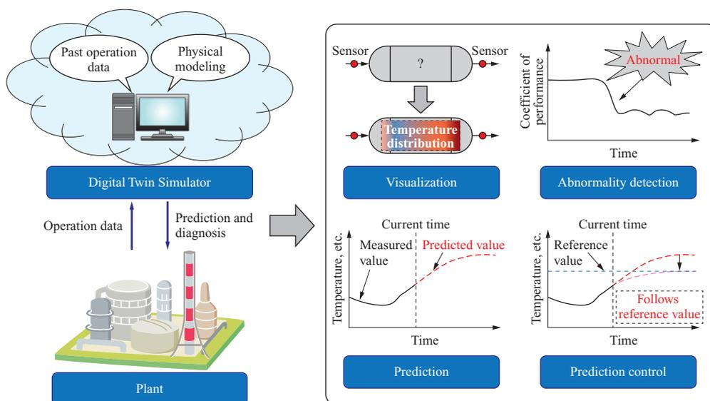
**Fig. 1 Conceptual schematic of Digital Twin Simulation**
