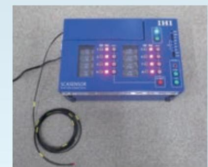
Smart Color Analyze Sensor is a concrete filling judgment device that uses an optical fiber and a digital RGB judgment device. The tip of the sensor is miniaturized and can be removed after judgment, leaving no foreign matter on the concrete structure.
