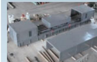
A vibration control device equipped on the suspension frames of offshore cranes. Reduces the shaking of offshore cranes caused by strong winds and waves and helps to improve the safety of hoisting loads.
