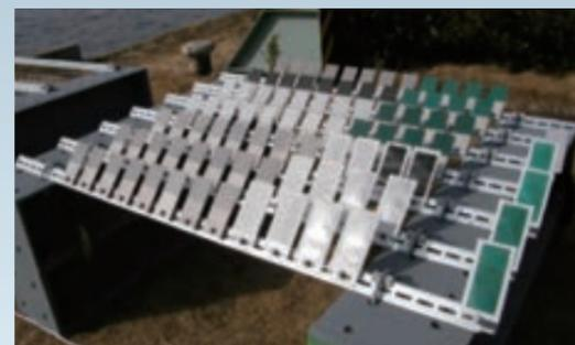
The prevention of corrosion-related degradation of bridges and gates is effective in the improvement of such structures' durability and reduction of LCC (lifecycle cost). IHI Infrastructure Systems conducts corrosion tests using various anti-corrosion methods and carries out R&D activities to improve anti-corrosion technology.
