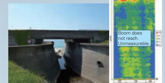
Concrete View uses spectrometry to make the concentration of chloride ions on the surface of concrete visible. Concrete View is anticipated to improve the efficiency of maintenance because it can predict areas which will deteriorate due to salt erosion, therefore can be used for position screening in detailed investigations, estimating repair area and used for incoming salt simulation.
