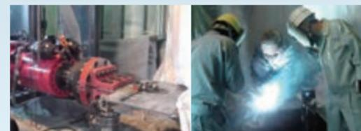
As a part of the repairs and reinforcement of social infrastructure predicted to become even more necessary in the future, we have used an actuator to reproduce the vibration assumed to occur during repair work on concrete slabs under real road conditions, in order to investigate welding material and conditions where defects would not easily occur.
