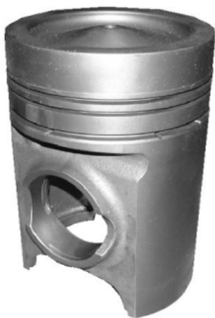
Figure4 Monoblock type piston
