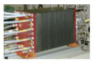
Prototype of a regenerative fuel cell
