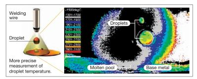
Droplet temperature measurement by high-speed video
