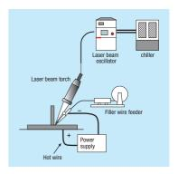
Schematic Diagram of laser hot wire welding process
