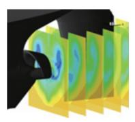
Flow velocity distribution behind semicircular duct (CFD analysis)
