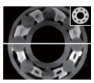
Neutron-beam and X-ray images (Top: rolling bearing before rotation, bottom: after rotation, upper-right insert: X-ray image)
