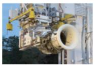
The *CF34-10A* undergoing ground tests (courtesy of GE)
