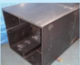
Mock-up test specimen for clean MIG welding of bridge structure
