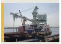
The new pneumatic unloader at Chiba Kyodo Silo Co., Ltd.
