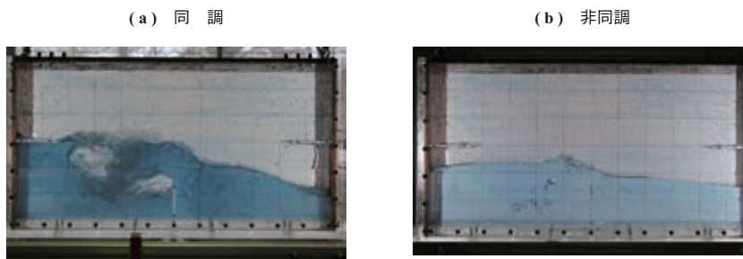
第6図 同調時と非同調時の貨液運動 Fig. 6 Liquid movement in resonance and non-resonance condition
