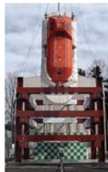
第 8 図 落下試験前後の状況 (2 回目) Fig. 8 Photograph before and after the drop test (2nd test)
