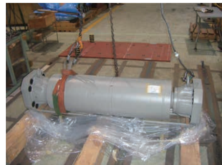
第 5 図 油圧ダンパ Fig. 5 Hydraulic damper that generates a damping force only in the extending direction
