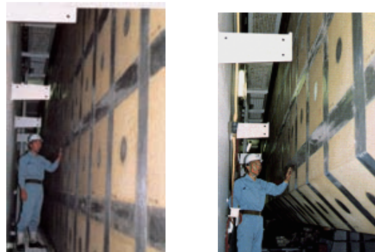
第 8 図 タンク外防熱材と船体間の歩路 Fig. 8 Walkway between inner hull and tank outside insulation
