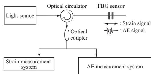
**Fig. 7** Schematic of simultaneous measurement for strain and AE using an FBG sensor
