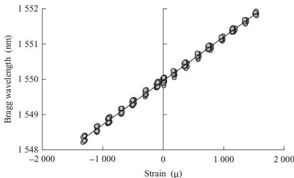
Fig. 3 Relationship between strain and Bragg wavelength
