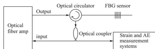
Fig. 5 Block diagram of measurement system using an FBG sensor and a fiber ring laser
