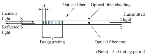
Fig. 2 Schematic of FBG principle
