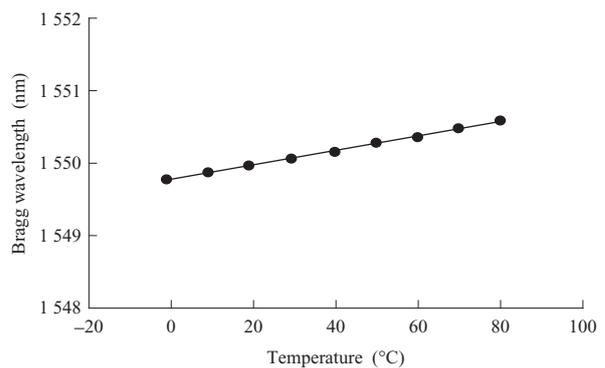
Fig. 4 Relationship between temperature and Bragg wavelength
