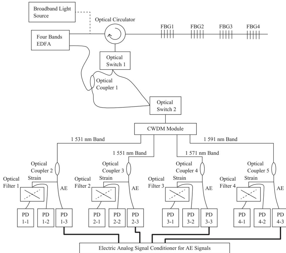
Fig. 8 Block diagram of the developed measurement system<sup>(8)</sup>
