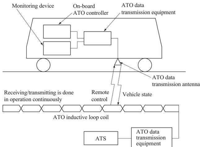
Fig. 5 ATO Data Transmission Equipment Configuration
