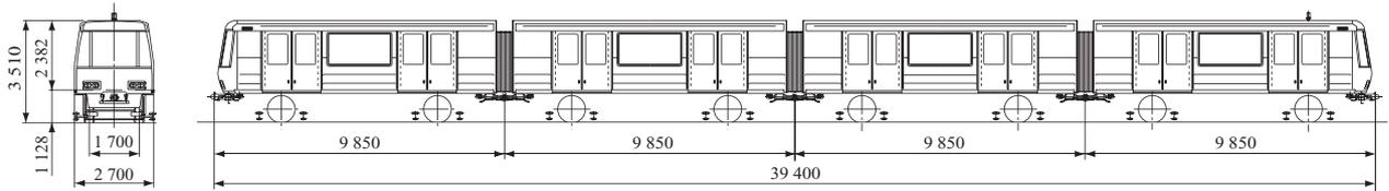
Fig. 7 APM Vehicle Set (Unit : mm)
