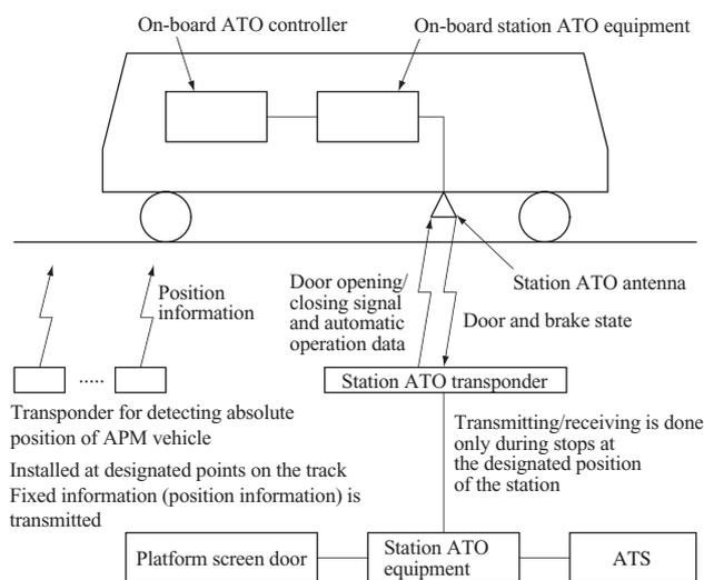
Fig. 6 Station ATO equipment Configuration
