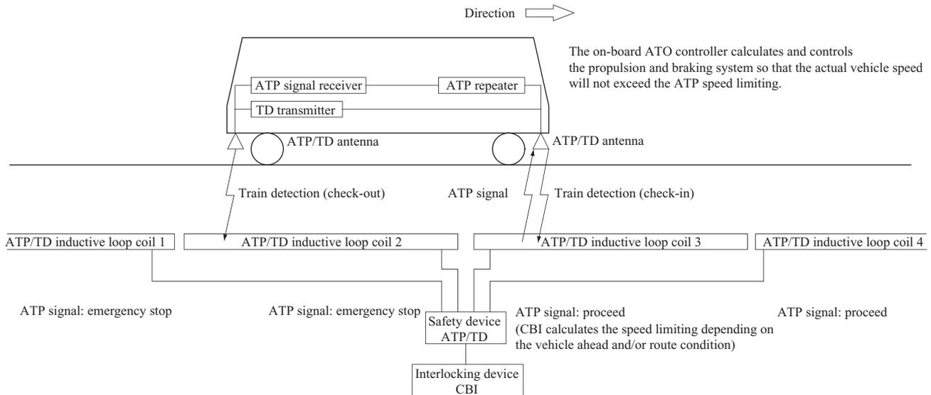
Fig. 4 ATP/TD Configuration
