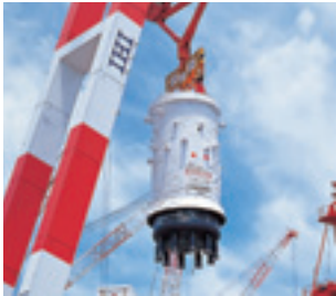
Reactor pressure vessel
