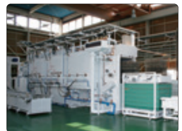
"V-presto" tunnel-type continuous vacuum carburizing furnace
