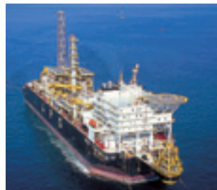
Floating LPG production, storage, and offloading facility
