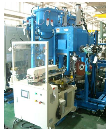
In-line heat treatment furnace
