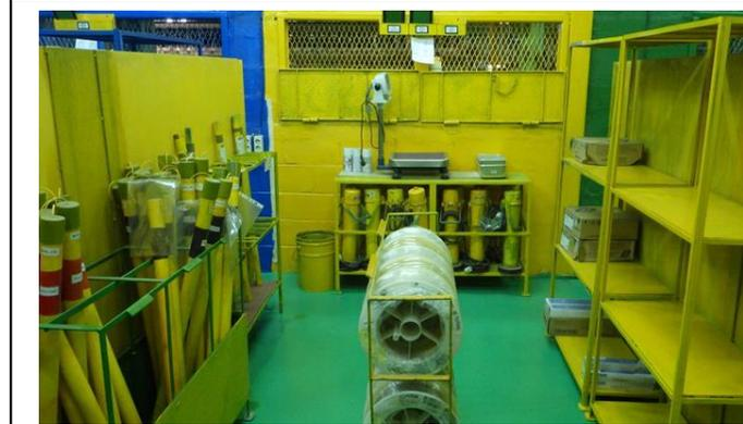
Management zone of welding material control room; P5 (Zone is color coded by welding materials)
