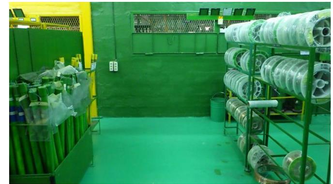
Management zone of welding material control room; P4 (Zone is color coded by welding materials)
