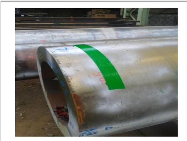
Color coding on materials (large diameter pipe)
