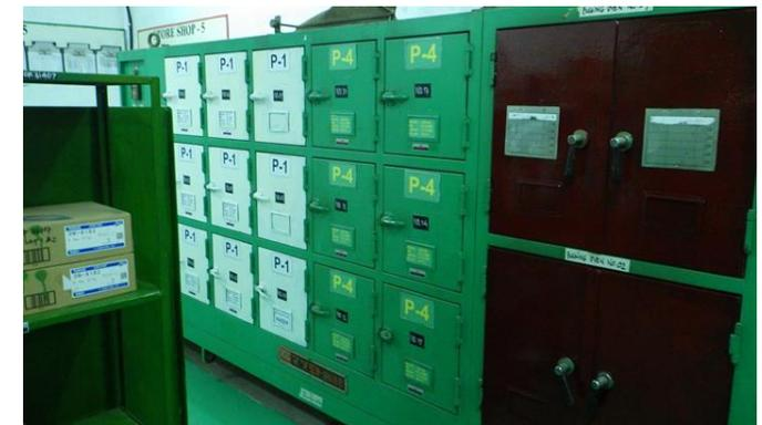
Color Coding for baking/ holding oven for SMAW (Shield Metal Arc Welding) material
