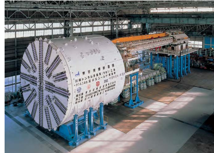
Large-diameter shield tunneling machines
