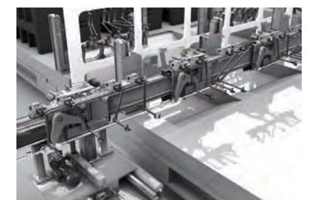
Retrofitting for conveyors between presses
